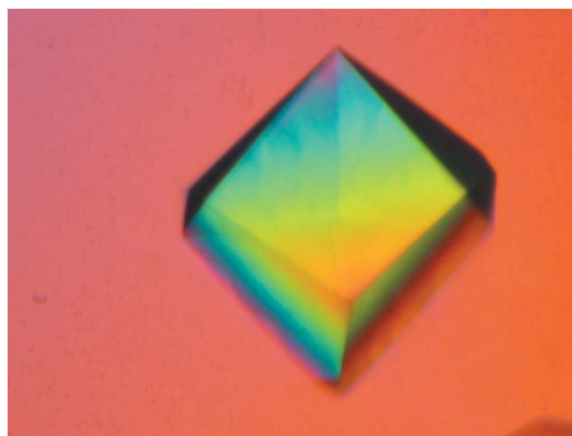
Figure 2 Crystals of MJ1225 grown by vapour diffusion at 293 K in 2.4 M ammonium sulfate, 2.8% PEG 400, 100 mM HEPES pH 7.5 with 11 mM FOS-choline 10 as an additive.
